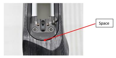
It's only the area that receive recoil and the areas that are under the back and front of the receiver that needs glass bedding. All other areas, especially the slanting one in the back of the receiver must be free of contact with the stock. Therefore, the glass bedding will be done in two steps. Step one on the back of the receiver and step two under the front of the receiver.
