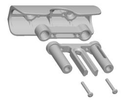
Put the spacer on the locking mechanism.
